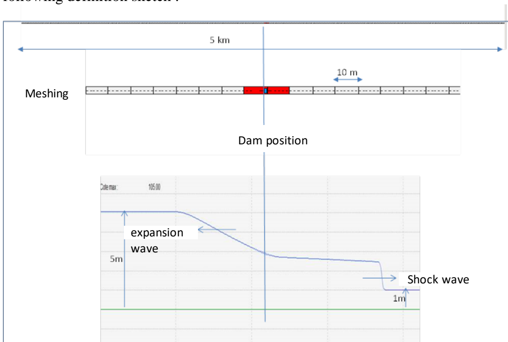
Figure 8 : definition sketch for the dam break problem
